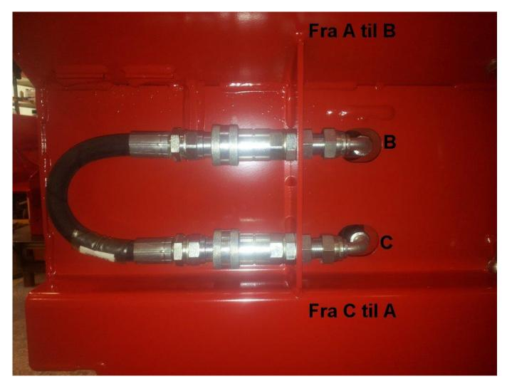
• The hydraulic hose that is connected between the quick couplings in the picture above is a bypass hose that must be used when the log rack is not in use.
